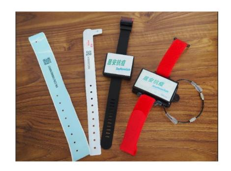
From first right to third right are BLE Bluetooth positioning electronic wristbands used for monitoring people under quarantine. The wristband in blue (first left) is the monitoring wristband using at the airport since March 19. All four wristbands are paired with the "StayHomeSafe" mobile app to detect and analyse changes in environmental communication signals to ascertain those under quarantine are staying in their dwelling places.
